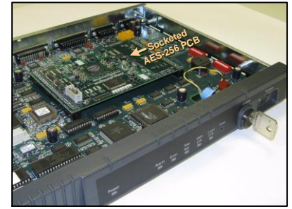
Internal view of Cipher X 7100 Unit showing AES-256 Crypto Processor PCB
